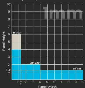
Vertical panels 48" and taller require Wind Clips at 24" on center Max
